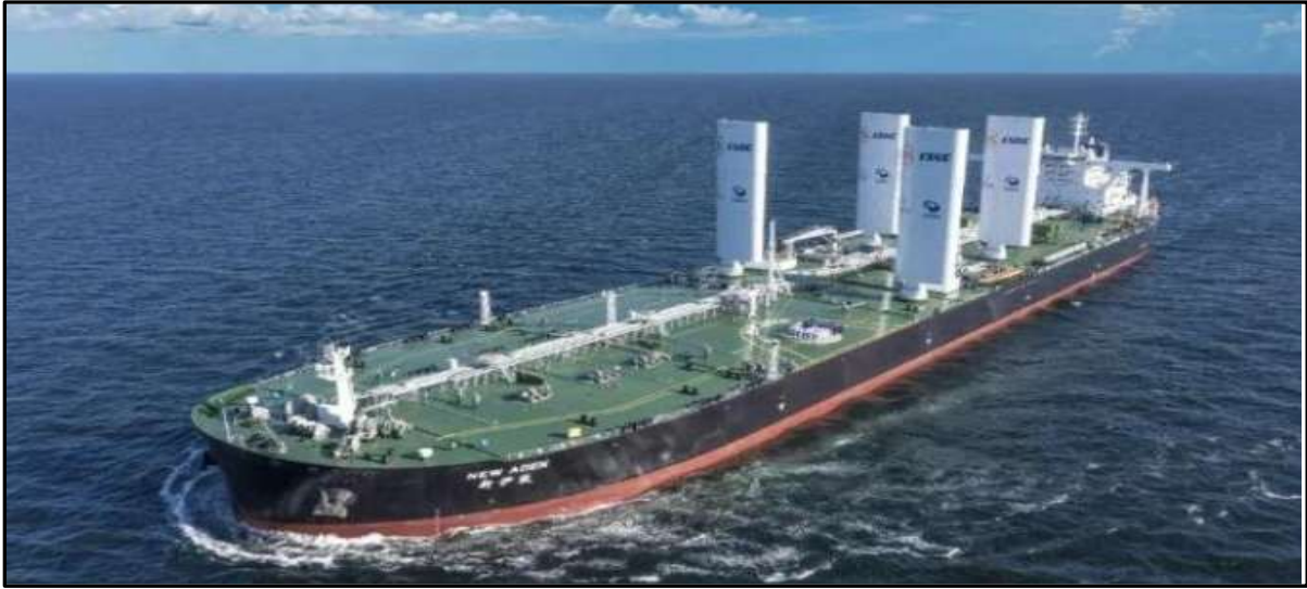
Figure 3. Wing sails placed on a tanker (The Maritime Executive, 2026)
