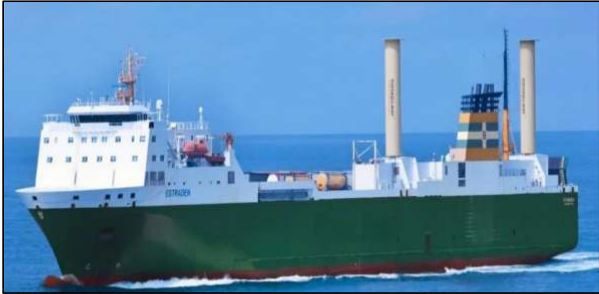
Figure 2. Flettner rotors on a Ro-Ro vessel (Spliethoff Group, 2026)
