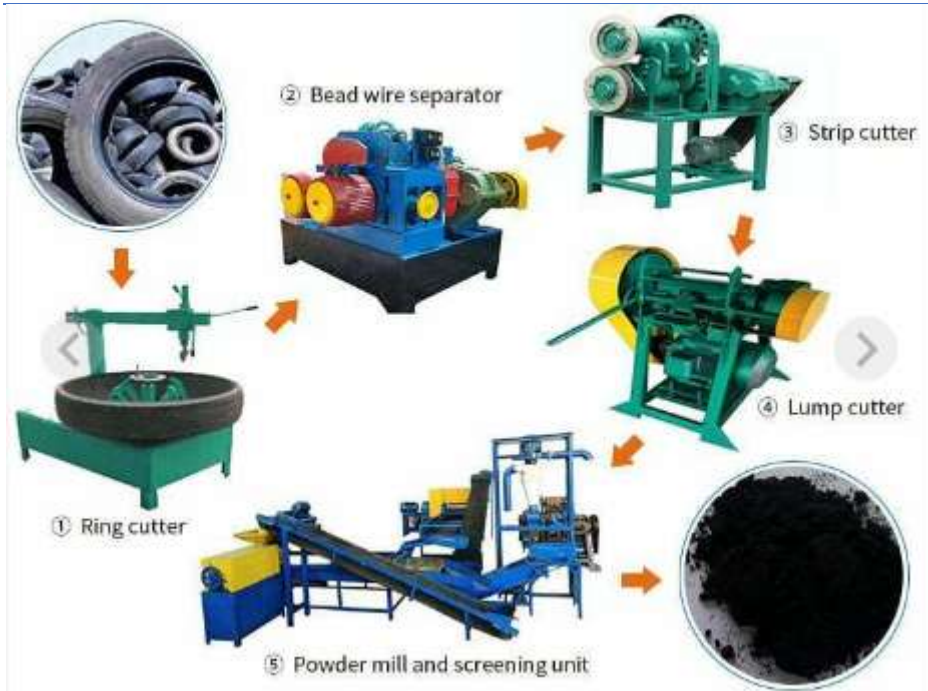
Fig.1 Mechanical milling and multi-deck screening equipment used for processing recycled tire rubber into fine powder
