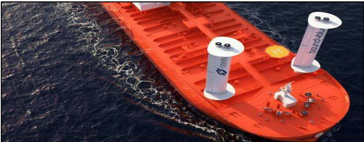
Figure 4. Suction wings installed on a Tanker (Odfjell, 2026)
