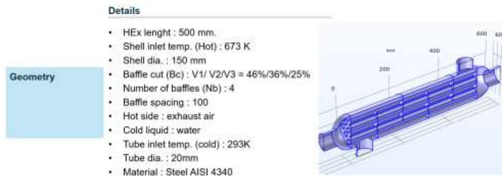
Figure 3. HEEx optimization iterations. add baffle, Bc:46%, 36%,25%
