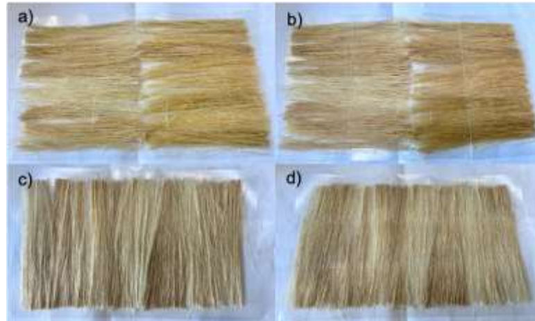
Figure 2: (a-b) 90° tape production, (c-d) 0° tape production
