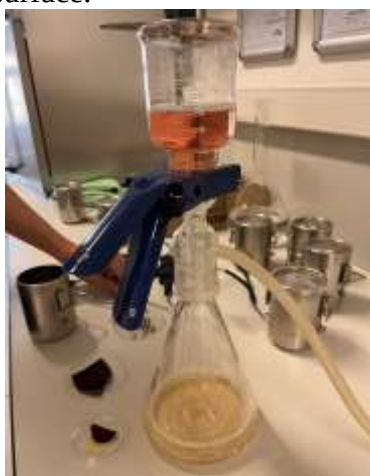
Figure 1. Vacuum filtration process for microfiber release
