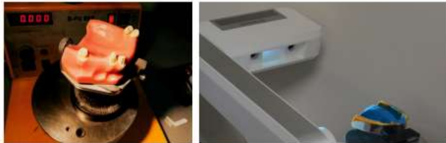
Figure 2. Standardized master model and laboratory scanning procedure using the laboratory 3D scanner.
