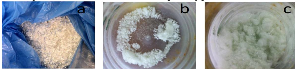
Figure 2. Views of E-glass fibers; (a) chopped E-glass fiber (PH 2 ) before fiber opening, (b) opened-up E-glass fiber (PH 2 ) after fiber opening, (c) opened-up E-glass fiber (PBT 2 )
